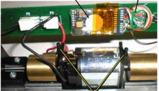
Remove (cutoff) unused post on motor supports
