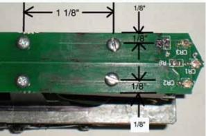
Solder the 2 brown wires from the module to the speaker Fasten the Speaker and Speaker housing together using 4 2-56 x 1/4" phillister heard screw and 2-56 ruts, Fasten speaker to cirecuit board with 2-56 x 3/16" screws. Do not use longer screws. They may touch the speaker
