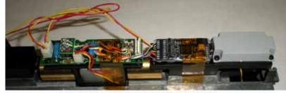
Fasten speaker and housing to frame with 4 screws. Fasten module to frame with Kapton tape or double sided foam tape. Gather wires and tape to circuit board with Kapton tape You are ready to go!
