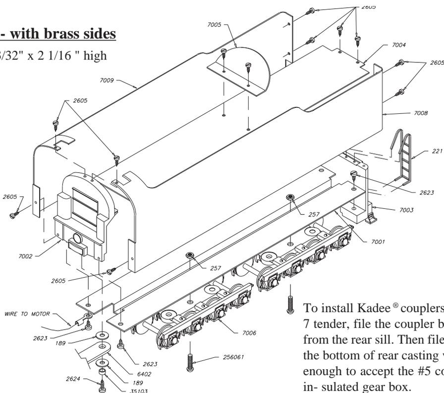
To install Kadee® couplers on the T-7 tender, file the coupler box detail from the rear sill. Then file a slot in the bottom of rear casting wide enough to accept the #5 coupler and insulated gear box.
