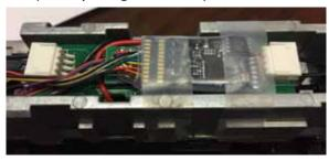
Place speaker on frame Hold in place with Kapton tape
