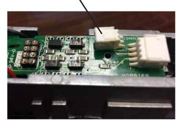
2 round solder spots after the slide lock removed
