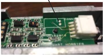
Solder motor wires
