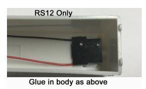
7. The RS 12 Headlight - glue the circuit board as photo above
