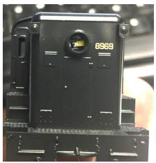
6. Glue or tape the circuit board with the LED centered in the light opening
