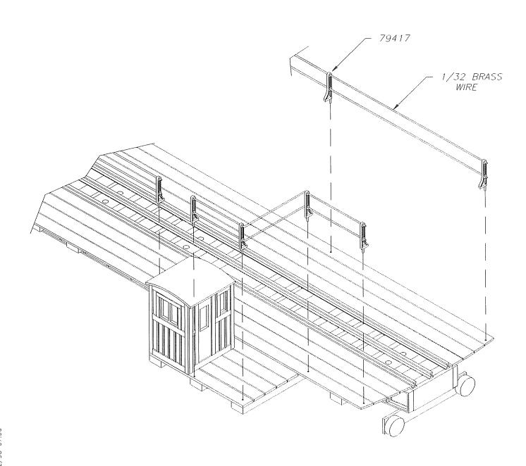
Locate and drill holes for tower in walks being sure to provide clearance for handrails.
