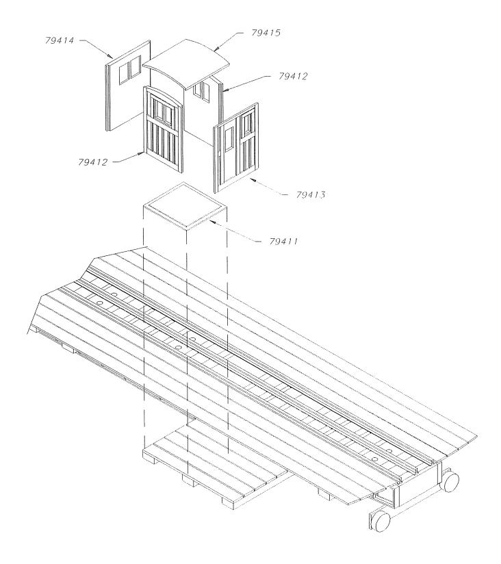
Drill 1/16" holes for handrail posts in walks above medium length and long ties. Assemble handrail posts to wire and glue to walks. Paint, install completed bridge into pit and ENJOY.
