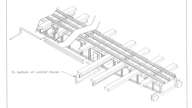
Install decking on bridge as shown. Glue in place. Raduis ends of decking to suit size bridge you are building.
