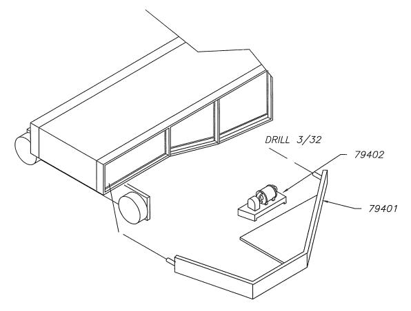
Note all wooden ties must have holes drilled for screws to prevent spliting.
