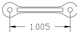
65000 Side rod, T-1, (brass) use 1720 side rod screw and 1721 main crankpin screw
