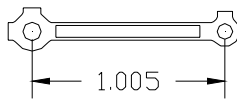
8712 Side rod, right, (brass) use 1720 side rod screw and 874 main crank spacer
