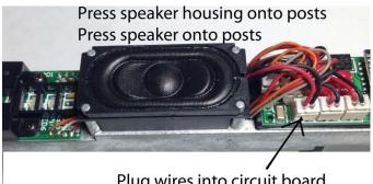
Plug wires into circuit board
